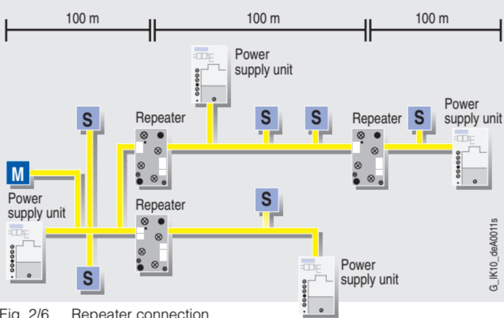
Fig. 2/6 Repeater connection
