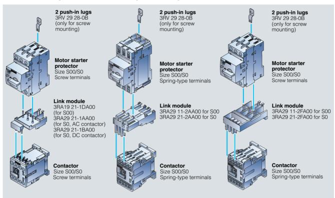
Left: 3RA2 load feeder with screw connection
