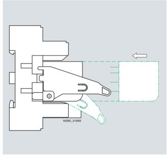
Important: The LZS:PT17021 and LZS:PT17024 ejection brackets of the coupling relays with plug-in relay are not status displays!
