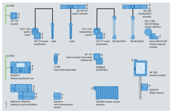
Due to its implementation of forward-looking technology, the "wave" device range is ideally suited for the retrofitting and modification of room control functions in existing buildings.
