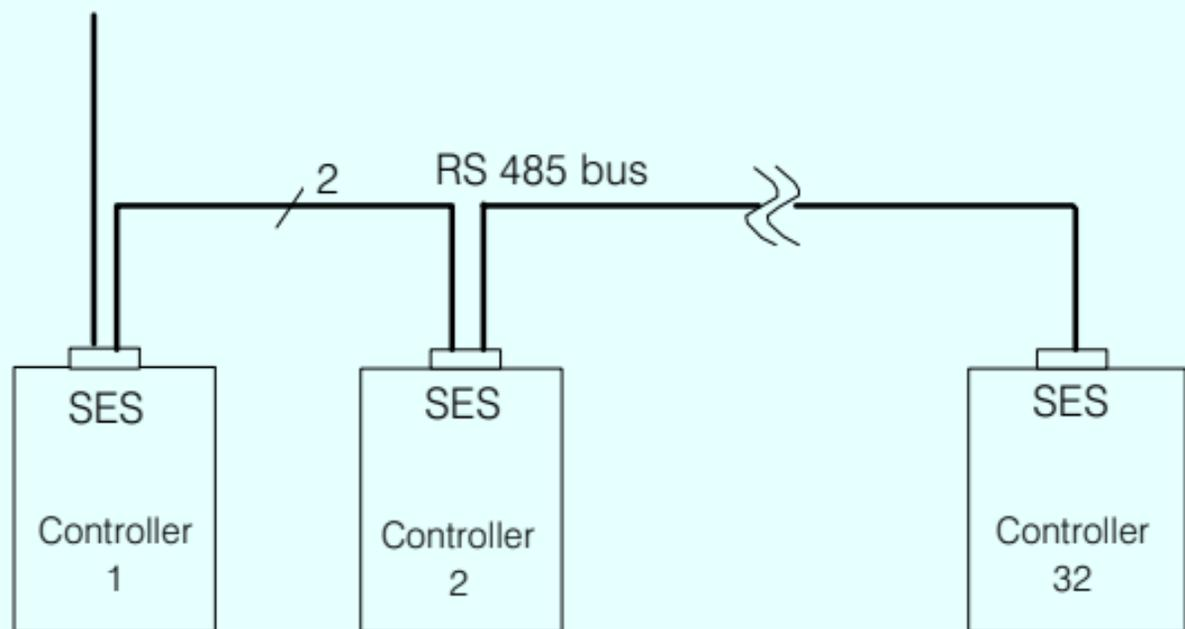
Fig. 1 Serial interface using RS 485
