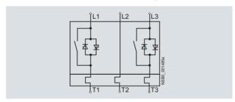
A bypass contact system and solid-state overload relay are already integrated in the 3RW40 soft starter and therefore do not have to be ordered separately.
