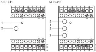
The voltage relays switch when the voltage falls below 90 % of the rated voltage. The 5TT3 411 relays serve to monitor a 1-phase infeed. 3-phase infeeds can be monitored using 5TT3 412 relays. These relays also offer asymmetry, reverse voltage and phase failure detection.
